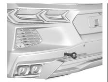
Install the tow eye into the socket and turn it until it is fully tightened.
