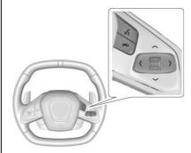
Press ≤ or > to access the cluster applications. Use the thumbwheel to scroll ∧ or ∨ through the list of available features. Press the thumbwheel to select. Not all applications will be available on all vehicles.
