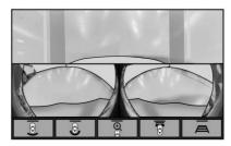
If equipped, a view of the area in front of the vehicle displays in the infotainment display. The display shows a front, top down view at the top and left and right front camera images on the bottom. The front view shows after shifting from R (Reverse) to a forward gear, or by pressing the camera button on the center console, and when the vehicle is moving forward slower than 12 km/h (8 mph).
