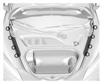
5. Release the four clips for the left and right outer covers.
