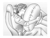
The driver frontal airbag is in the centre of the steering wheel.
