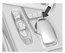
To activate My Mode, Weather, Tour, Sport and Track Mode, turn the Driver Mode Control (DMC) knob on the center console to make a mode selection. When a mode is selected, an indicator will illuminate in the instrument cluster and remain illuminated.
