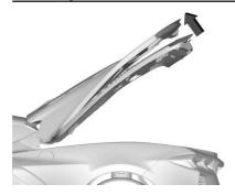
To provide more access to the engine or trunk areas, the hatch/trunk can be manually pushed up for additional travel. Do not apply excessive force.
