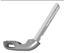
The mechanical key can be used to open the vehicle and hatch/trunk if power to the vehicle is lost. See Hatch (Boot)  $\Rightarrow$  20.
