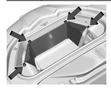
If equipped, the vehicle has a convenience net to be used for small loads. Attach the net to the hooks of the storage area. The net should not be used to store heavy loads.
