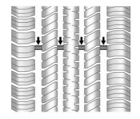
Tread wear indicators are one way to tell when it is time for new tyres. Tread wear indicators appear when the tyres have only 1.6 mm (1/16 in) or less of tread remaining. See *Tyre Inspection* ⇒ 272 and *Tyre Rotation* ⇒ 272 for additional information.
