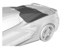
Hold until the tonneau cover is completely closed. A chime will sound, a DIC message will display, and the turn signals will flash once.
