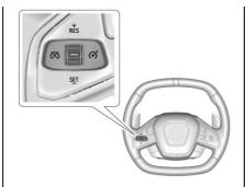
ኛን : Press to turn cruise control on or off. A white indicator comes on in the instrument cluster when cruise is turned on.
