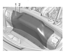
5. Remove the rear compartment access panel screws (2) and panel (1).
