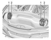
Remove the four lift off bracket bolts (2) to remove the brackets (1).
