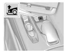
To use the Front Lift System, press the button on the center console to raise or lower the vehicle. This feature can be operated at speeds up to 38 km/h (24 mph) when the engine is running. The system functions based on the vehicle's state or operating mode:
