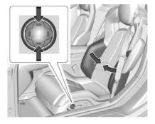
If equipped, press and hold the control upward to increase or downward to decrease the side bolster support.
