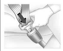
Push the latch plate into the buckle until it clicks. Pull up on the latch plate to make sure it is secure.
