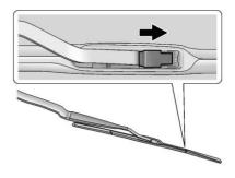
Lift up on the latch in the middle of the wiper blade where the wiper arm attaches.
