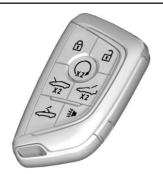
**立**: Press to lock both doors and the fuel door. The indicators may flash and/or the horn may sound on the second press to indicate locking. See "Remote Lock, Unlock, Start" under *Vehicle Personalisation*
