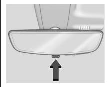
Pull the tab to turn on the display. Push the tab to turn it off. When the display is off, the automatic dimming function is active. Adjust the mirror for a clear view of the area behind the vehicle while the display is off.
