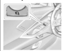
If equipped, press a to power fold the mirrors. Press again to unfold.
