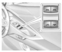
Press to lower the midglass. To provide wind block, the midglass will not lower completely. The midglass will also lower automatically when lowering the convertible top.
